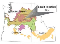
environmental and subsurface data. Scientists will inject 1,000 tons of CO2 (the amount a typical coal-fired power plant emits in a few hours) about 2,700 feet underground and monitor it for 14 months. The project has been permitted by the Washington Department of Ecology and funded by the U.S. Department of Energy and other private companies.
