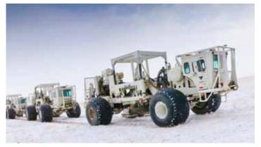
Seismic vibration trucks move together along the grid stopping at intervals to create soundwaves.
