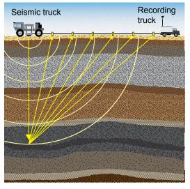
Seismic trucks generate sound waves which are reflected back and detected by the sensor array.
