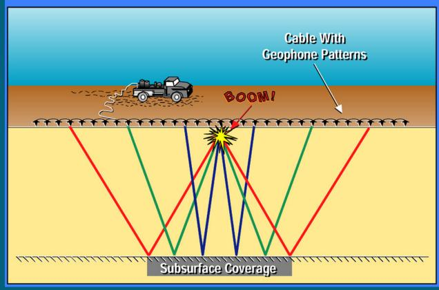
To improve data quality and reduce noise in the data each subsurface point is multiply sampled to increase what is called 'fold'.
