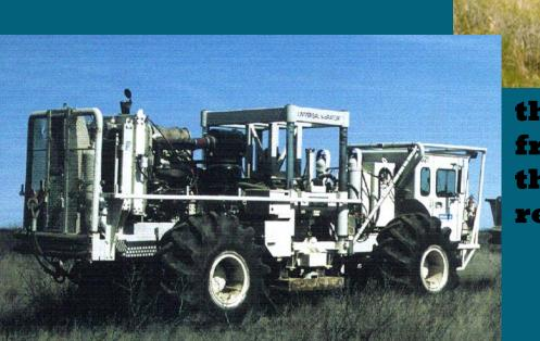
the amount of high frequency energy put into the ground to provide more resolution in the final data.
