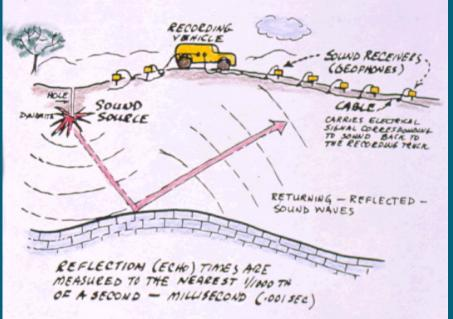
BY CAREFULLY MEASURING AND RECORDING THE REFLECTION TIMES THE GEOPHYSICIST CAN DETERMINE HOW DEEP - EVEN NOW THER-VARIOUS ROCKS ARE ...
