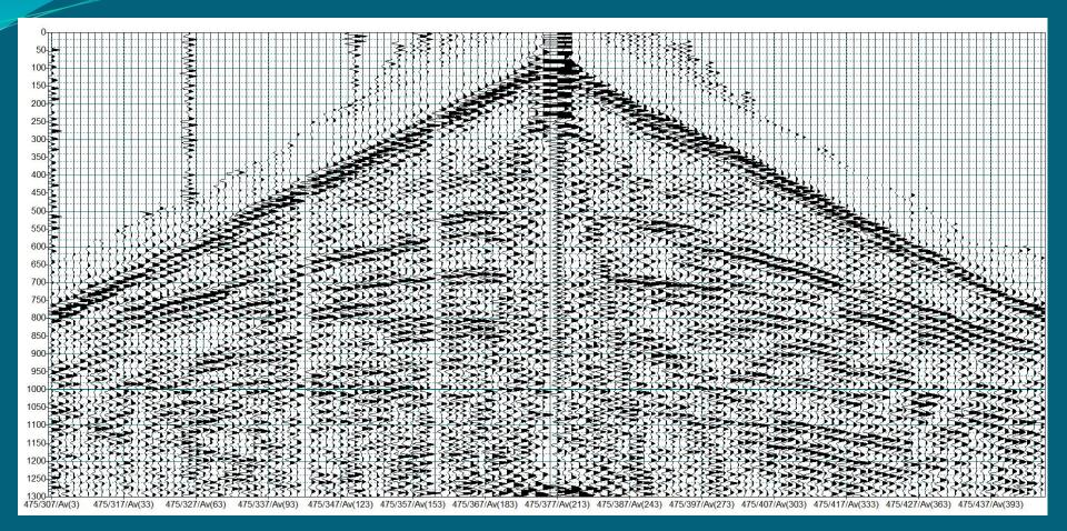
Seismic data consists of a series of recorded wiggle traces that describe a set of echoes from interfaces between rock layers in the subsurface that have different rock properties.
