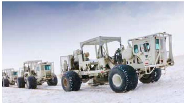
*Seismic vibration trucks move together along the grid stopping at intervals to create soundwaves.*
