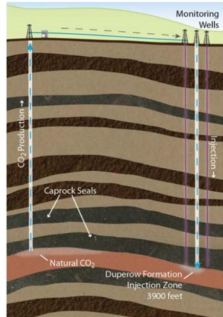
**Figure 1:** Cross-section of subsurface showing the role of caprock layers, like anhydrite, in securing  $\text{CO}_2$  deep underground.
