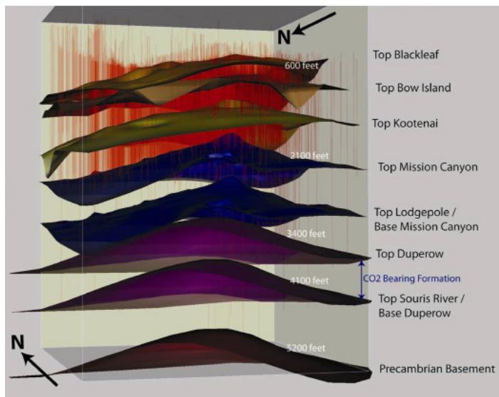
**Figure 2:** Geologic model depicting subsurface layers of interest at Kevin Dome. Red lines show wells drilled in various formations as of 2009. Updates to this model are ongoing.
